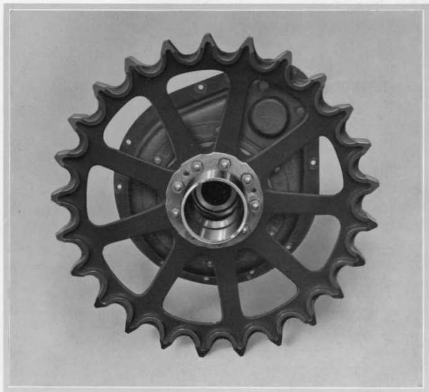
This shows the Drive Sprocket and the case that encloses the final drive gear and pinion.
