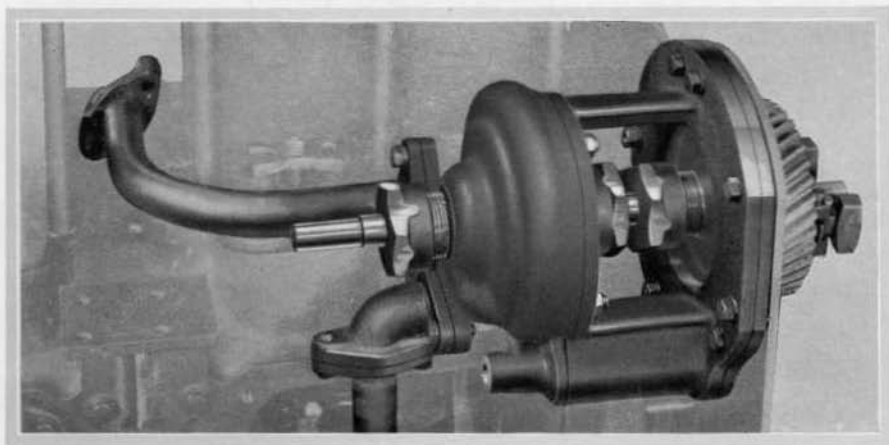
A close-up view of the Water Pump Unit.
